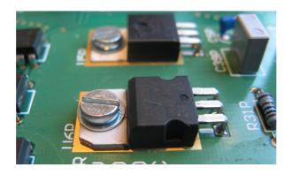
As exception to the 'normal' mounting order, I propose to wait with mounting the 4 opamps and the 2 microcontrollers: complete all mounting except these 6 IC's and the XLR connectors. We can now first test the correct operation of the power supplies before inserting these ICs, avoiding the risc to blow them due to some earlier mistake. So, without the 4 opamps and 2 microcontrollers U1D and U2D, you connect the two transformers, and power them up. Please check the following voltages:
